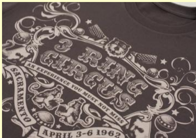
Discharge printing on Black shirts, using 150/inch, 48 micron, S-thread
