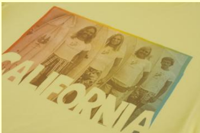
Printing with 180/inch, 48 micron, S-thread
