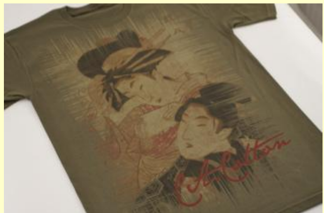
Both shirts printed with 330/inch, 30 micron, S-thread
